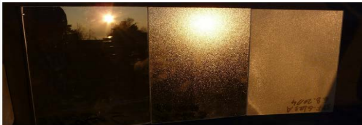
Fig. 3 photographic picture of the sun reflected by three different glass types. left: flat float glass, middle: rolled glass with a slightly structured surface, right: rolled glass with macroscopic pyramidal structure.
