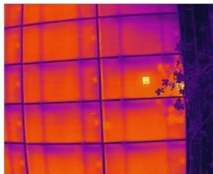
Corrosive misaligned bus bar of SPV module
