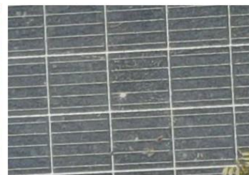
Corrosive misaligned bus bar of SPV module
